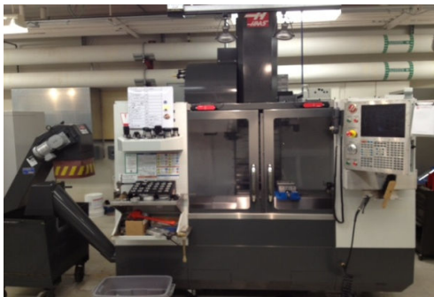
Fig. 3 CNC HAAS Vertical Machining Center, Model VF2TR
