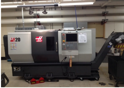
Fig. 2 CNC HAAS Turning Center, Model ST20
