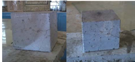
Fig. 3 Concrete specimens subjected to 800°C
