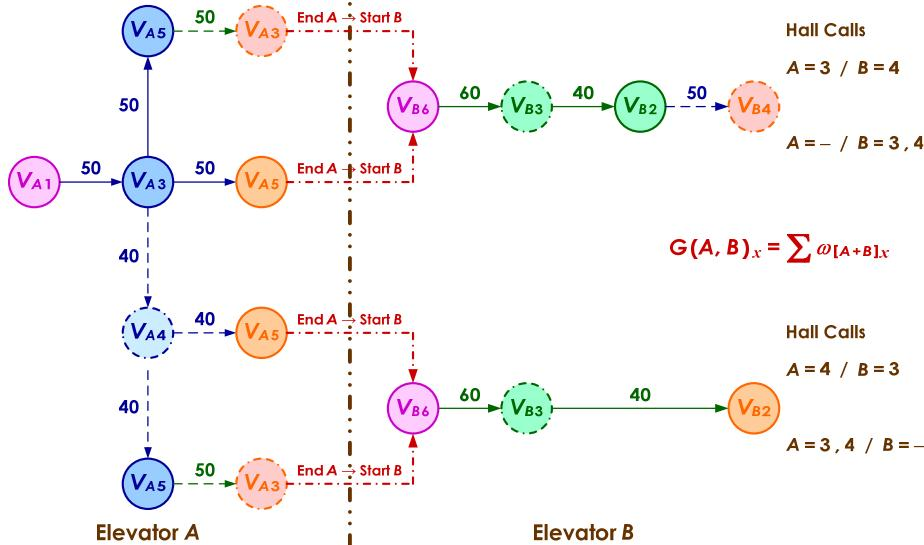
Fig. 1 Weighted graph showing all travel path combinations
