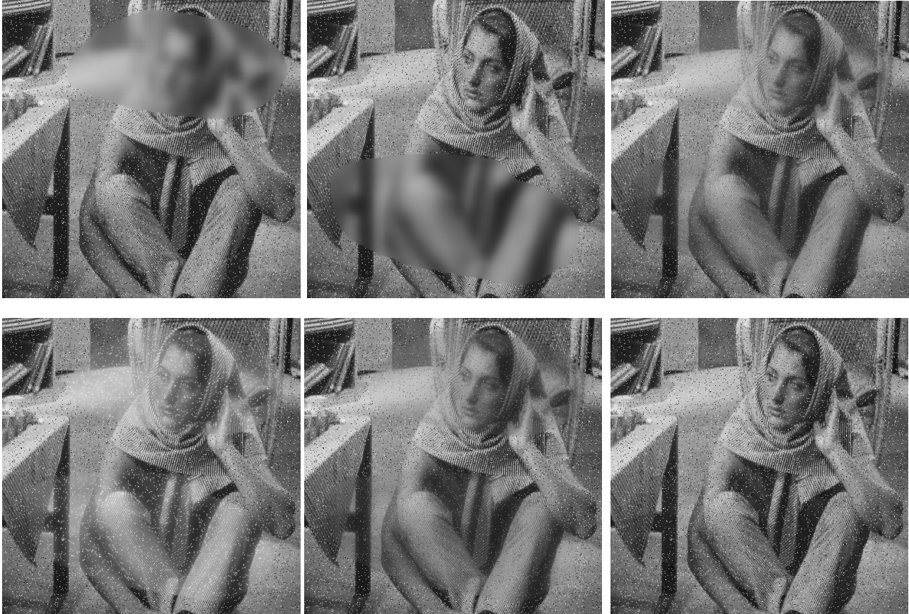
Fig. 3 Fusion results, the original image corrupted by the salt and pepper noise and partial blurring. Top: input image X (the original image with added noise and a blurred segment, left), input image Y (the original image with added noise and another blurred segment, middle), fused image F using averaging (right). Bottom: fused image F using ratio pyramid decomposition (left), fused image F using the PCA decomposition (middle), fused image F using DWT domain fusion (right)
