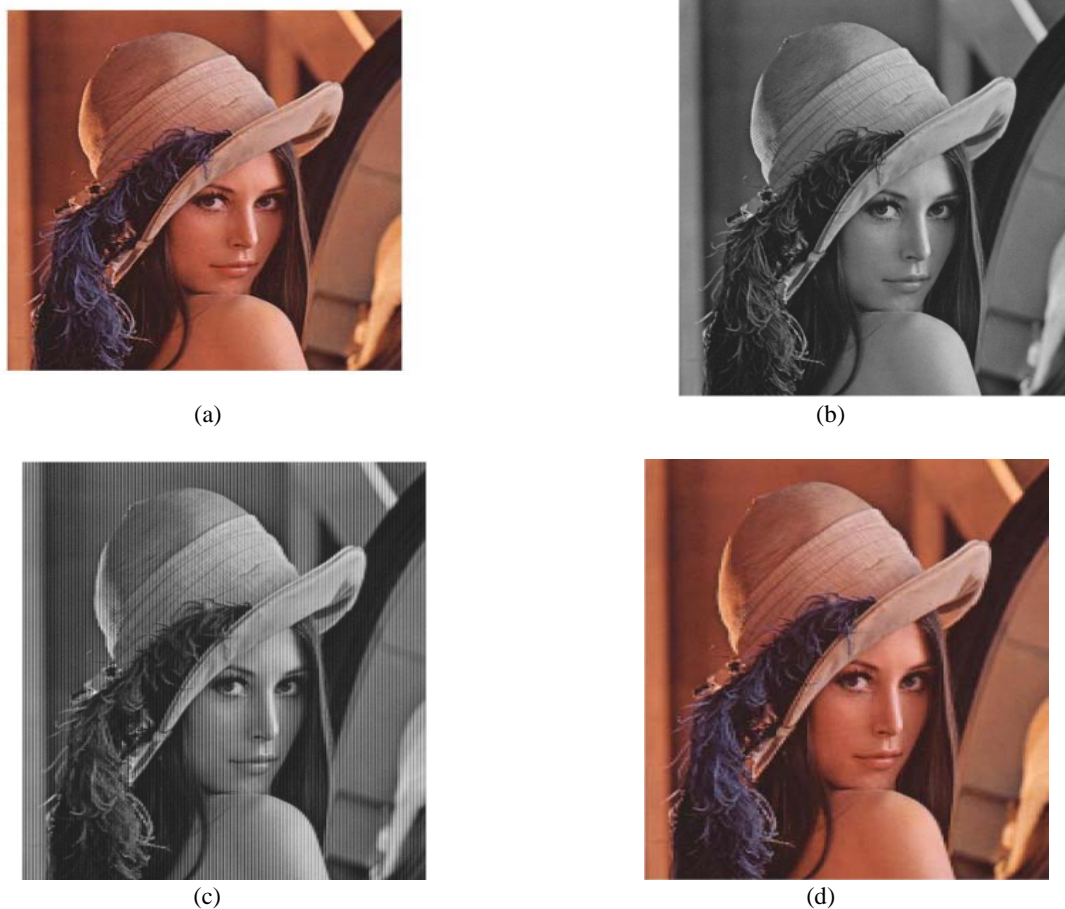
Fig 3 (a)Original colour image (b)-grayscale image (c) compressed image (d)-reconstructed colour image
