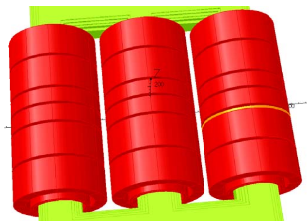
Fig. 8 Model of the faulty transformer TO294-22kV with axial short circuit (orange)
