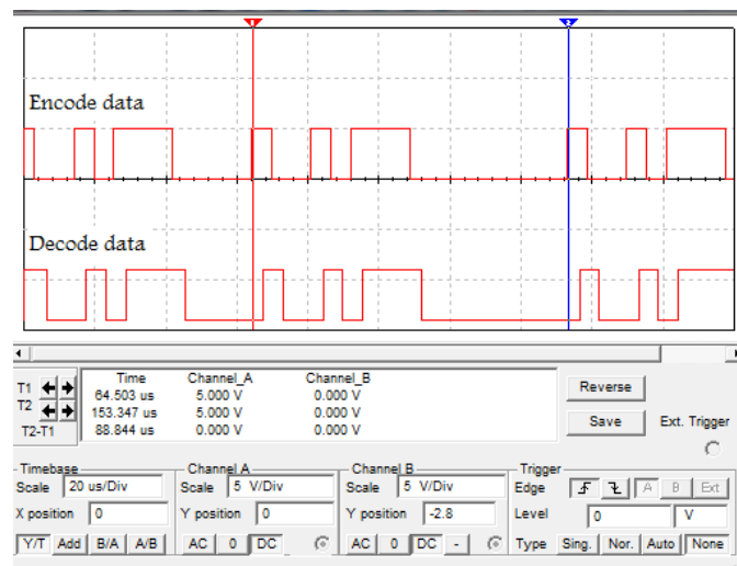
Fig. 9. The required time for sending 8 bits of data (88.844 \mu s / 90kbps), and the ability of the receiver to decode these encoded data at this speed
