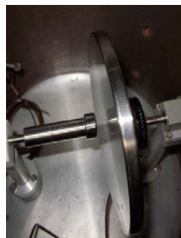
Fig. 2 Stainless Steel electrodes: Rogowski/plane electrode configurations
