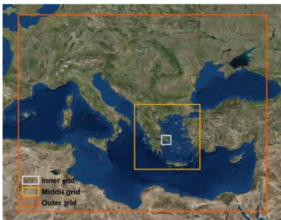
Fig. 5 The system of nested grids used for the CAMx simulations
