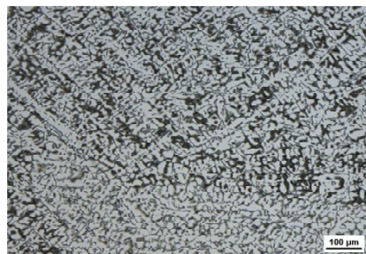
Fig. 1 The \alpha -phase in secondary AlSi9Cu3 cast alloy, as-cast state. Optical microscope, etch. H_2SO_4
