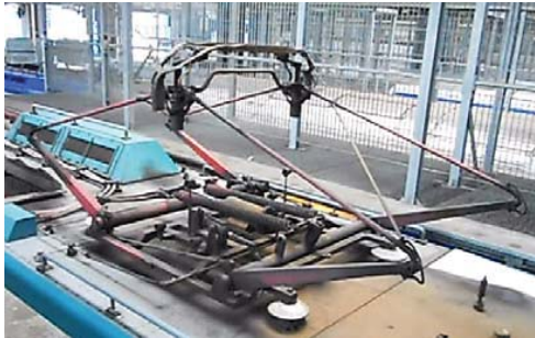
Fig. 1 A picture of the railway pantograph under consideration (courtesy of Trenitalia)
