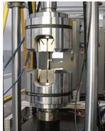
Fig. 5 Hydraulic fatigue test machine [1]
