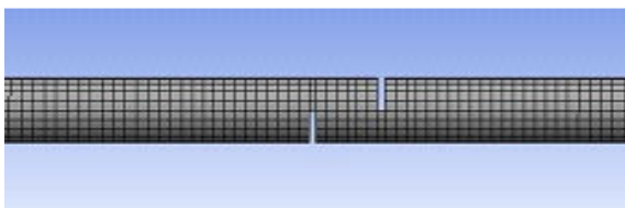
Fig. 2 Hexdominant mesh of flow geometry
