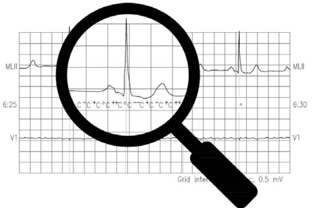
Fig. 2: The differences between consecutive ECG signals define letters from alphabet \Sigma = \{C^0, C^+, C^-, C^{++}, C^{--}\}
