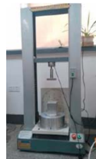
Fig. 3 The test equipment used for the calibration of FTS
