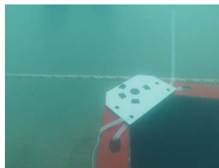
Fig. 10 Image showing the use of Agisoft Pgotoscan Pro markers for better automatic alignment in processing (Photograph Felix Pedrotti)
