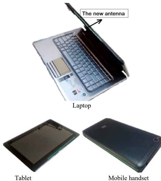
Fig. 6 The antenna mounted on different terminals
