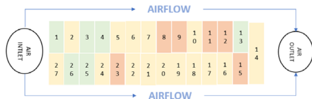
Fig. 15 Grading results of 27 cells in system planar diagram, in which green indicates grade A, yellow indicates grade B, red indicates grade C
