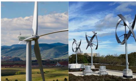
Fig. 12 Horizontal vs. Vertical Axis Wind Turbines
