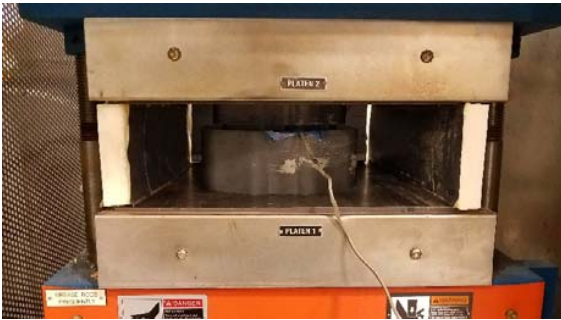
Fig. 8 Mold assembly loaded in heated press
