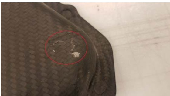
Fig. 15 Carbon fiber valve cover defects
