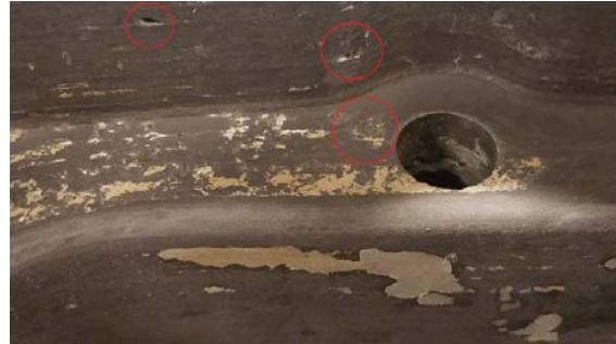
Fig. 10 Chipping defects of the mold surface
