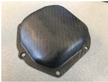
Fig. 9 Completed carbon fiber valve cover
