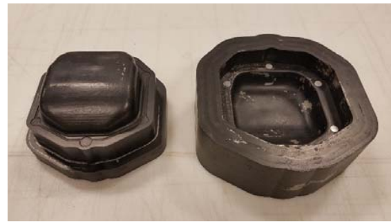
Fig. 5 Completed 3D printed composite compression mold
