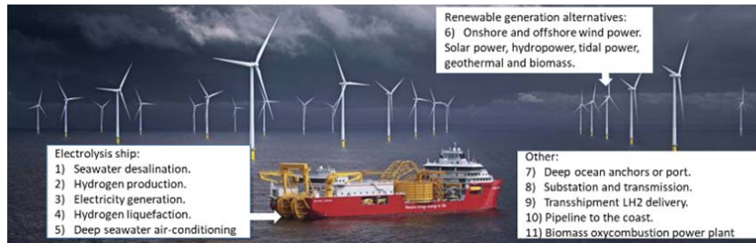
Fig. 1 Electrolysis ship components
