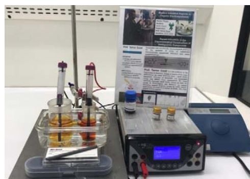
Fig. 2 The controlled-potential organic electrosynthesis cell design
