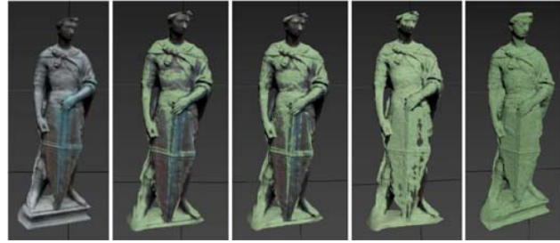
Fig. 3 Simulated ageing of a bronze statue of Saint Giorgio at 5-year intervals
