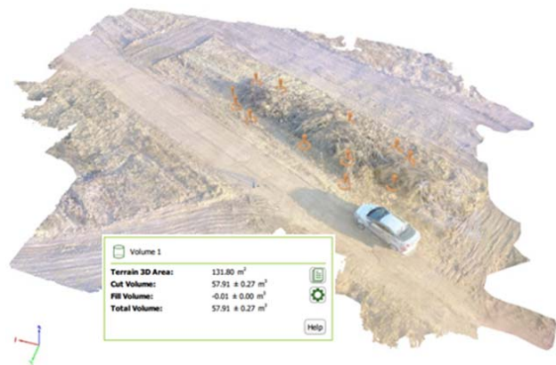
Fig. 7 Models of test area from UAV during test trials in Israel (April 2017): using images from DJI Mavic Pro
