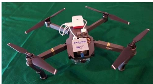
Fig. 2 The fire detection sensor on PI-Zero W mounted on DJI Mavic
