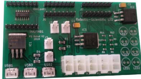
Fig. 6 Electronic board designed to provide different voltages
