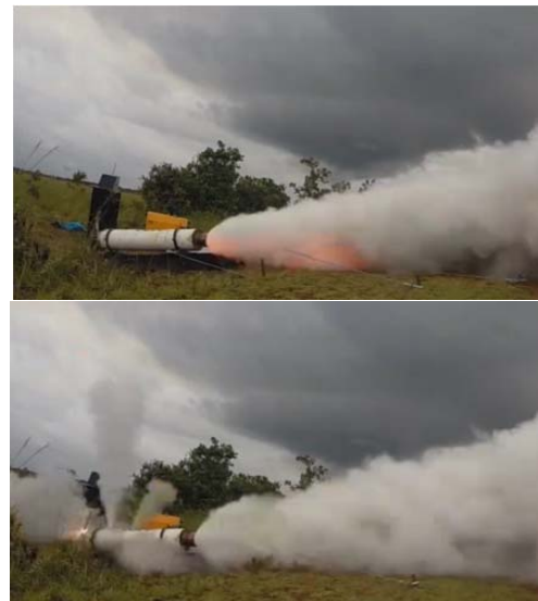
Fig. 3 Illapa 1 engine test and failure [10]
