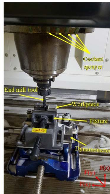
Fig. 1 Experimental setup for the milling test
