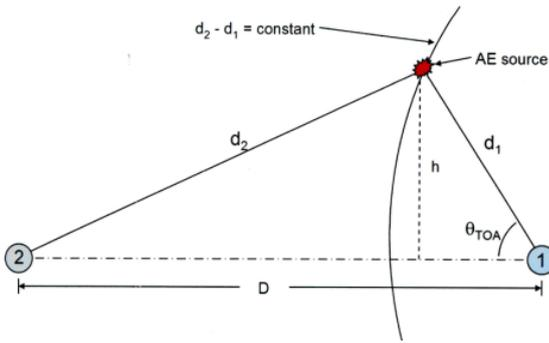
Fig. 5 D location on an infinite plate [2]
