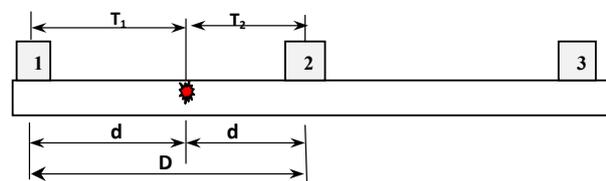
(c) Hits sequence, time difference measurement  $\Delta t = T_2 - T_1$
