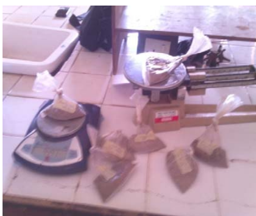
Fig. 6 Electronic Scale, Weighing Balance and Weighed Soil Sample
