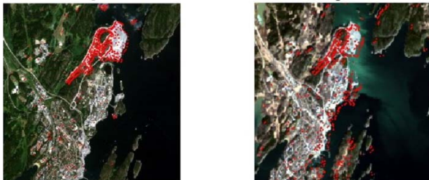
Fig. 10 The detected changed pixels shown both in Sentinel-2 and Landsat-8 in approximately four months gap
