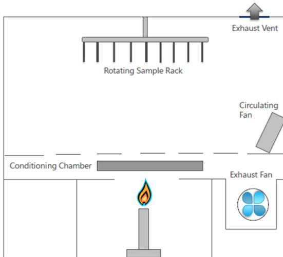
Fig. 1 Atmospheric fume chamber for gas fade test
