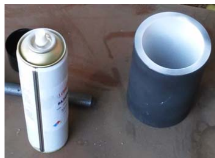
Fig. 1 Graphite crucible coated with boron nitrite
