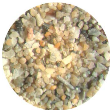
Fig. 1 Microscopic image of Bushehr calcareous sand
