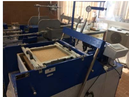
Fig. 3 Large scale direct shear tests on sandy soil
