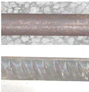
Fig. 3 Bars used as reinforcement [16]
