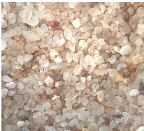
Fig. 1 Optical microscope image of the Firouzkouh sand
