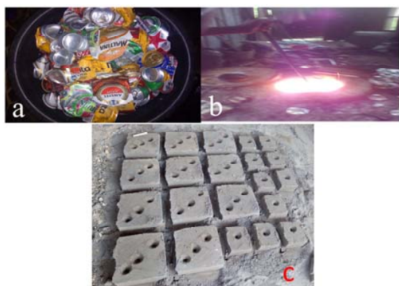
Fig. 1 Materials and casting of HEA (a) Drink cans, (b) stirring of the alloy mix and green sand mold prior to pouring of the melt
