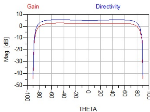
Fig. 6 Gain and directivity for 2.6 GHz
