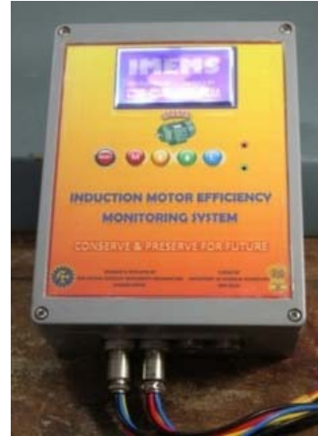
Fig. 3 View of the developed MPM Node
