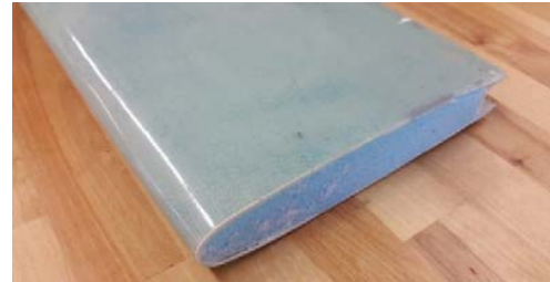
Fig. 4 Complete wing core with fiberglass skin
