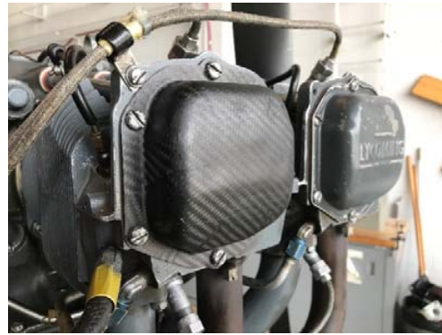
Fig. 14 Test fitting of carbon fiber valve cover
