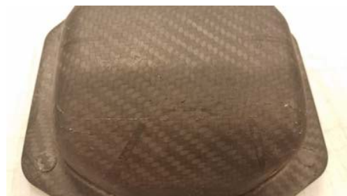
Fig. 9 Surface defects caused by mold surface cracking
