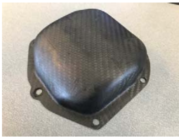
Fig. 7 Completed carbon fiber valve cover
