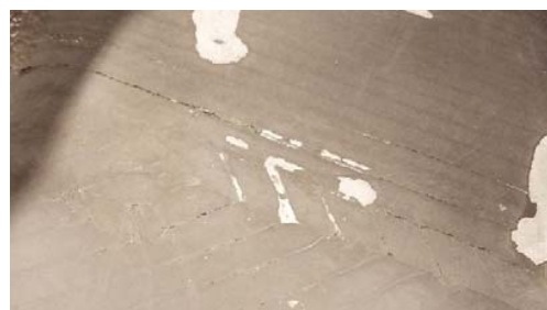
Fig. 11 Mold surface cracking between beads
