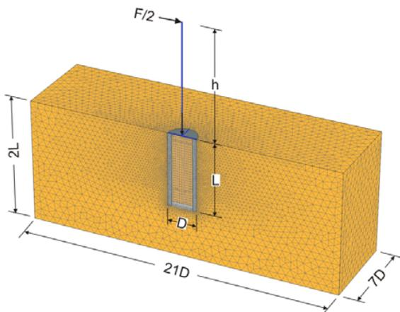
Fig. 3 Finite element mesh of the pier foundation
