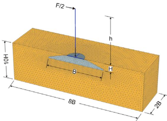
Fig. 2 Finite element mesh of the shallow foundation
