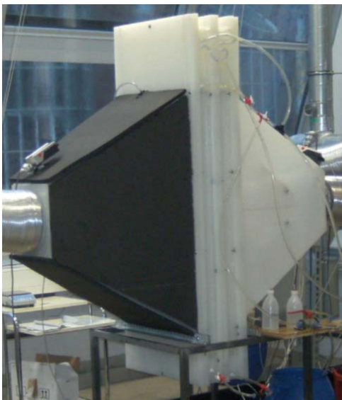
Fig. 4 Assembly of the absorber with air diffusers
