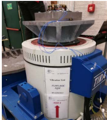
Fig. 7 DOC installed on the TIRA shaker for Out of Plane Test
