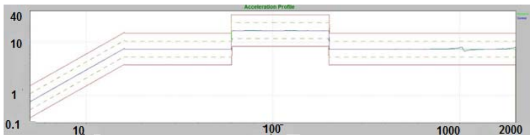
Fig. 10 DOC EQM HLSS Measured levels –Acceleration vs Frequency
