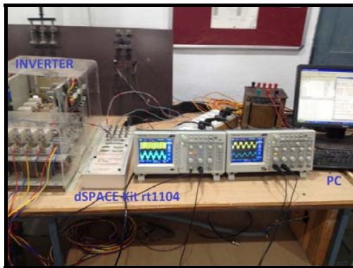
Fig. 43 Zoomed portion of Hardware Setup
