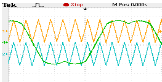
Fig. 7 Modulating reference and level shifting carrier signals: CSVPWM
