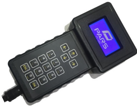
Fig. 3 Calibration device used to input parameters into VU
