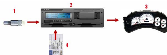
Fig. 1 Components of the tachograph system
