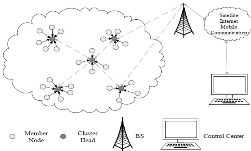
Fig. 1 Typical WSN logical hierarchy diagrams
