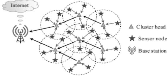
Fig. 2 Wireless Sensor Network model
