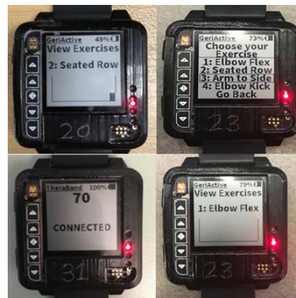
Fig. 4 (b) Snapshot of states of TheraBand application: a) specific exercise type; b) choosing an exercise; c) connected; and d) specific exercise type
