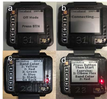
Fig. 4 (a) Snapshot of TheraBand application states: Off (a); Connection (b); View of band color (c); Initiation of Exercise (d)
