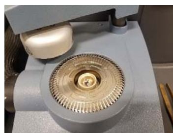
Fig. 8 Specimen loaded in DSC's chamber
