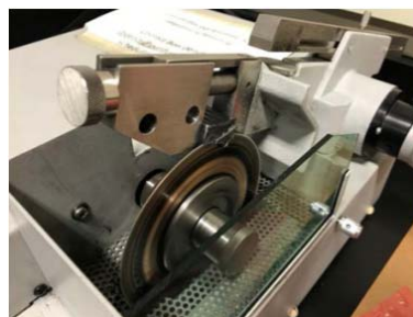
Fig. 2 Specimen sectioning using a precision diamond saw
