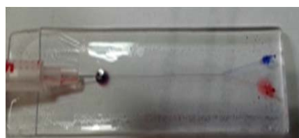
(b) Mixing behavior of Y micro-mixer after filling with colors
